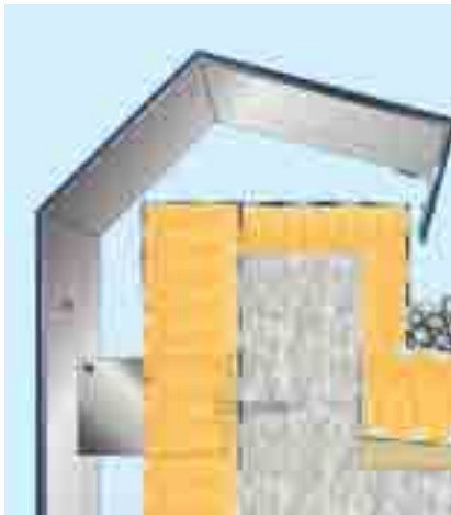
Upper end of panel - vertical section
