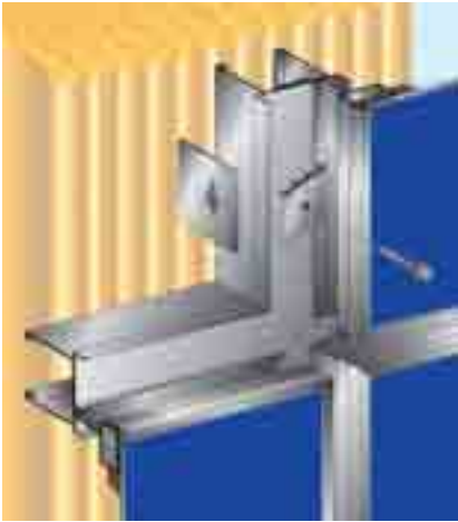
ALUCOBOND® panels framed with bonded edge sections
