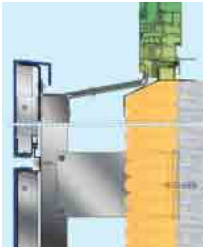
ALUCOBOND® window sill with internal drainage - vertical section
